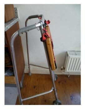
To fold the tray away, one pulls up the <u>back</u> of the tray. The Velcro loops then slide up the legs of the Zimmer frame, until the tray lies flat against the legs. The tray is then held in the folded-up position by its weight and the pressure from the straps in front, helped by the slight backwards slope of the Zimmer frame
